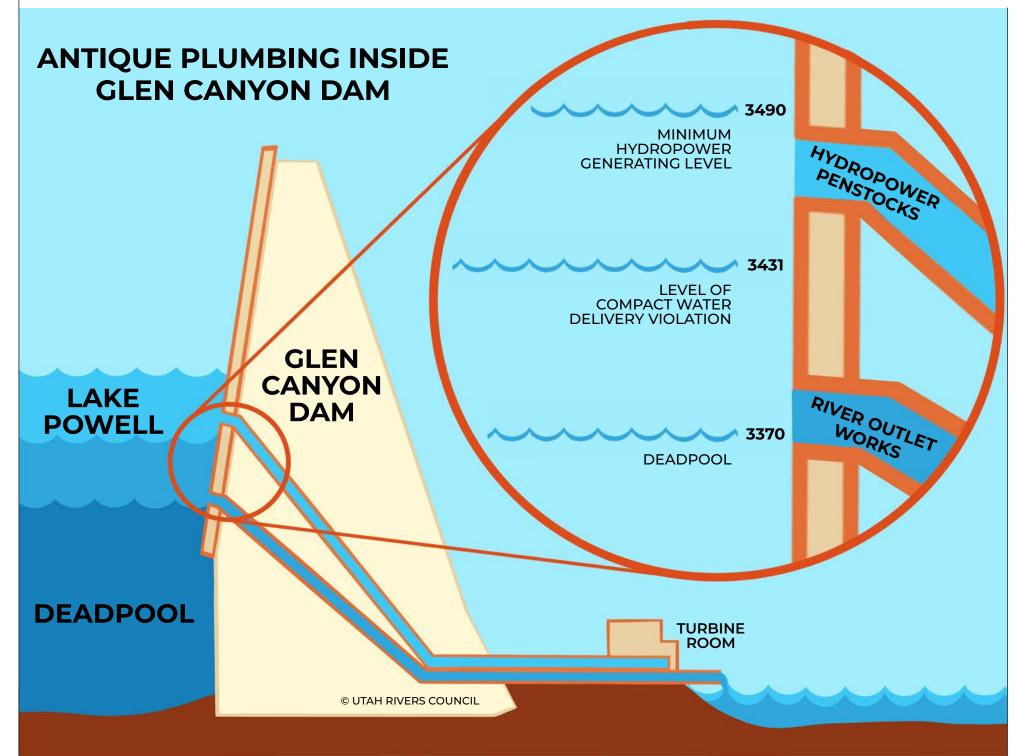
The River Outlet Works were not designed to permanently deliver large quantities of water,<sup>19</sup> as their main role is to supplement water releases from the reservoir when the hydropower releases are not adequate. In the dam's lifetime, the River Outlet Works have only been used when the dam first filled, during the
